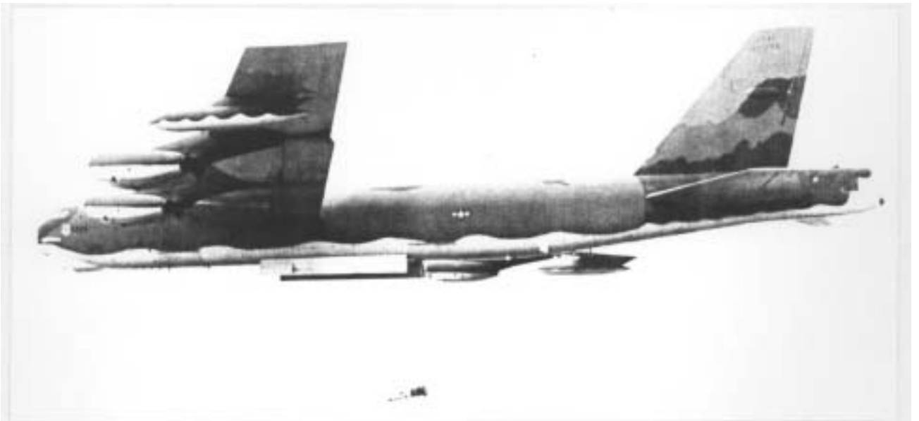
Fig. 7: "Mines Away!" A Strategic Air Command B-52G releases a sea mine. (USAF Photo, 1985)
